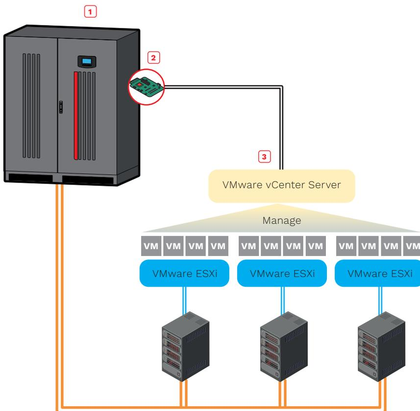
NetMan 208 should be used for managing Esxi hosts and vCenter servers, enabling you to manage your virtual network to perform shutdown or live migrations of active virtual machines as well as shutdown of physical hosts with delay and priority.
