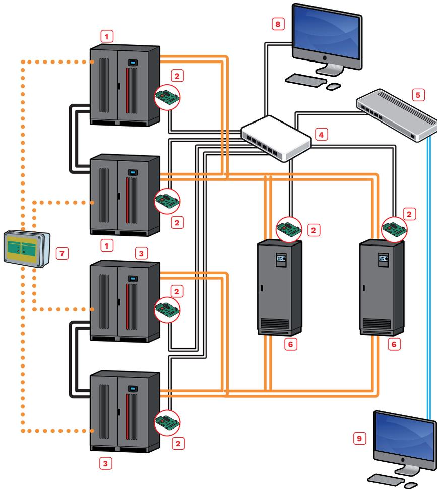
The FULL version of PowerShield<sup>3</sup> software should be used for managing setups with several UPS installed in parallel and each UPS must have a NetMan 208 board installed.
