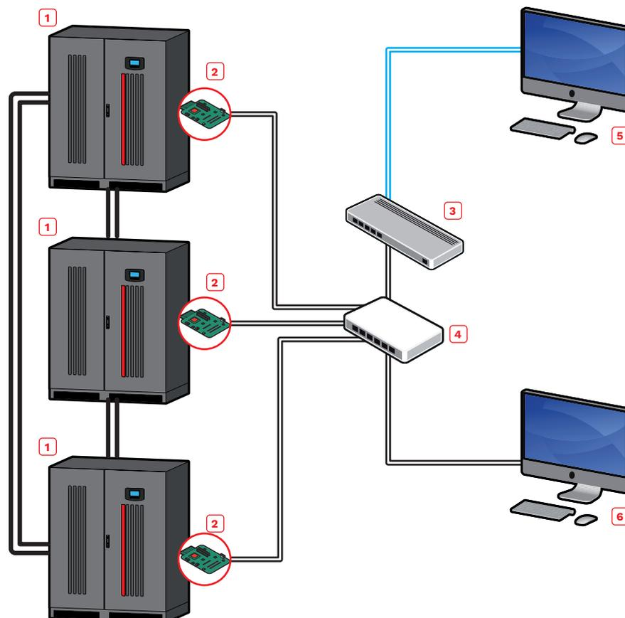
The FULL version of PowerShield<sup>3</sup> software should be used for managing setups with several UPS installed in parallel and each UPS must have a NetMan 208 board installed.
