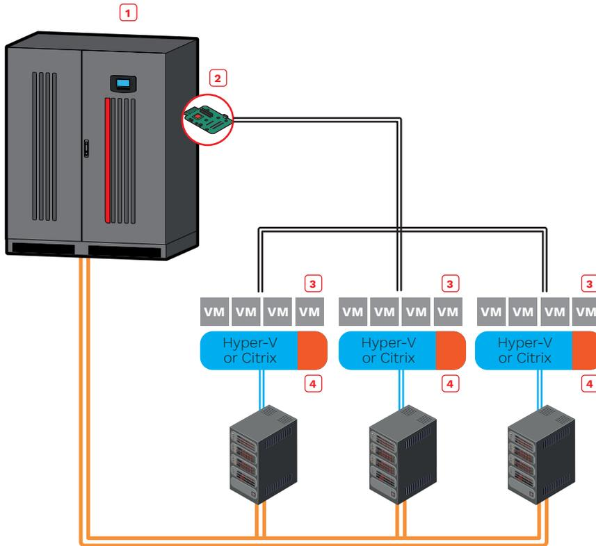
Powershield<sup>3</sup> software should be used for managing setup with UPS, a specific script to shut down the virtualised system must be used, UPS must have a NetMan 208 board installed.
