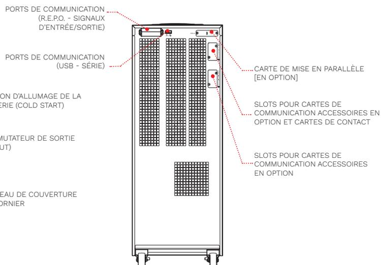
PORTS DE COMMUNICATION (R.E.P.O. - SIGNAUX D'ENTRÉE/SORTIE)
