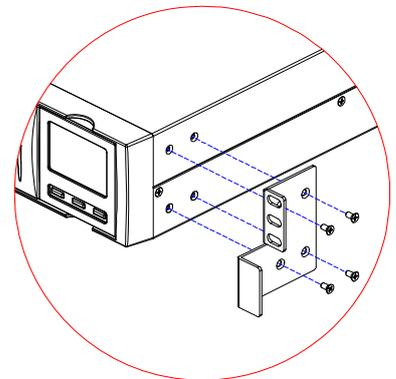
**NOTE:** Given the heavy weight, the use of support brackets is mandatory during rack installation (guide with L-shaped support). For the same reason, it is recommended that the UPS and battery box be installed in the lower part of the rack cabinet.
