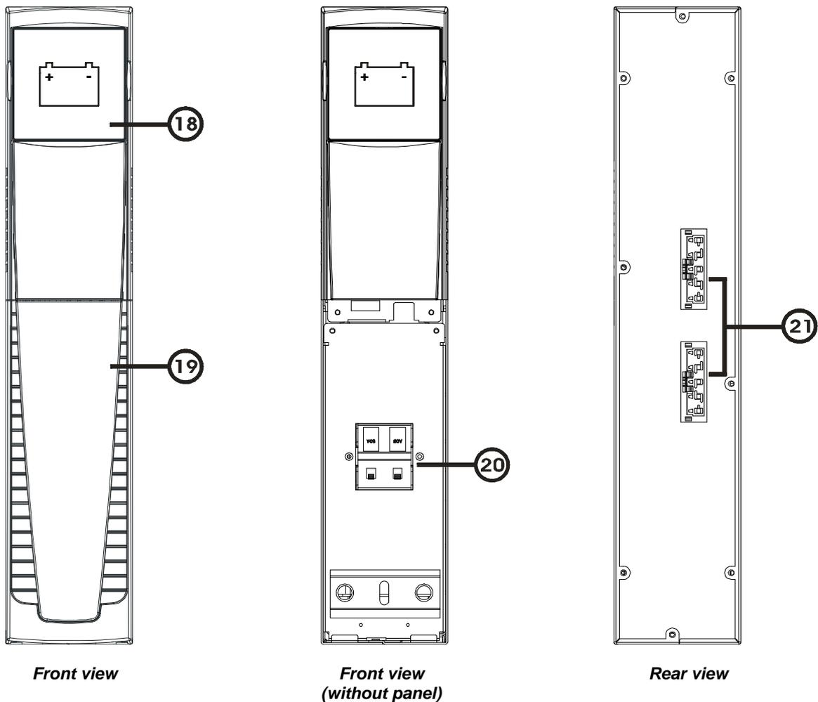
**18** Extractable/ rotatable battery box plate
