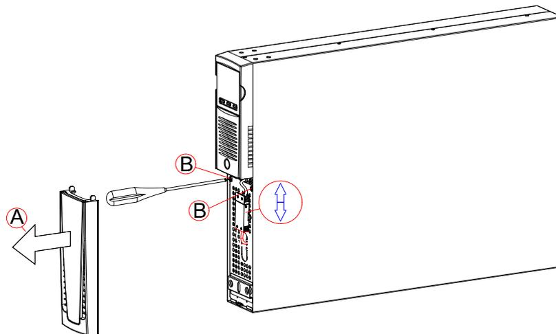
3. Remove the battery pack's retention panel carrying out the operations shown in the figure below.
