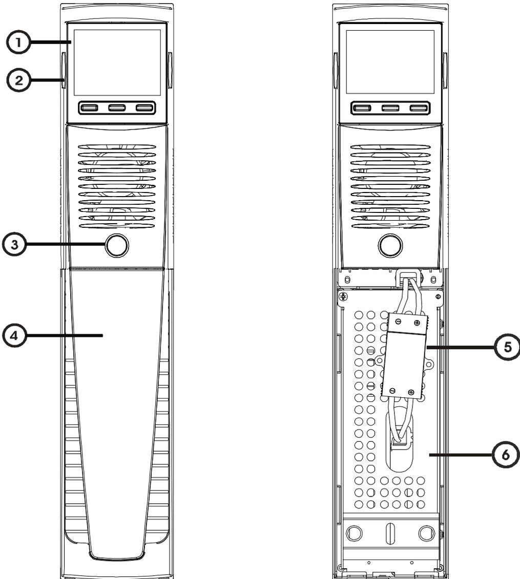
① Extractable/rotatable display plate
