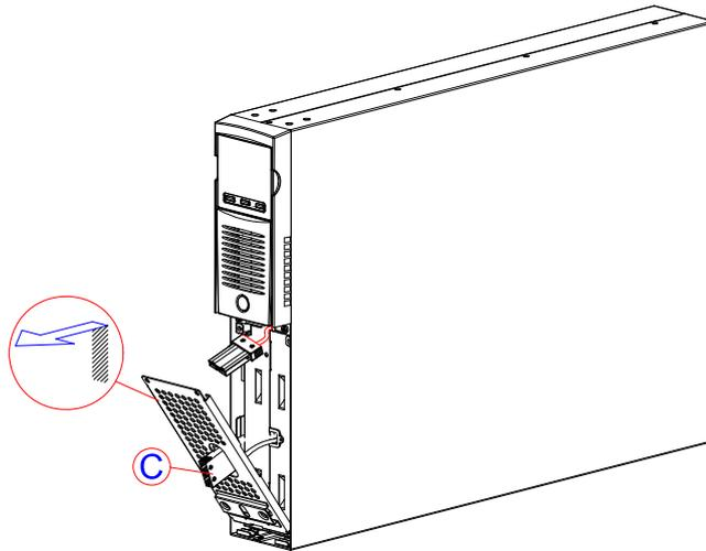
4. Slip off the battery pack pulling it towards the outside, as shown in the figure below. Be careful when extracting and lifting up the battery pack as it is heavy.
